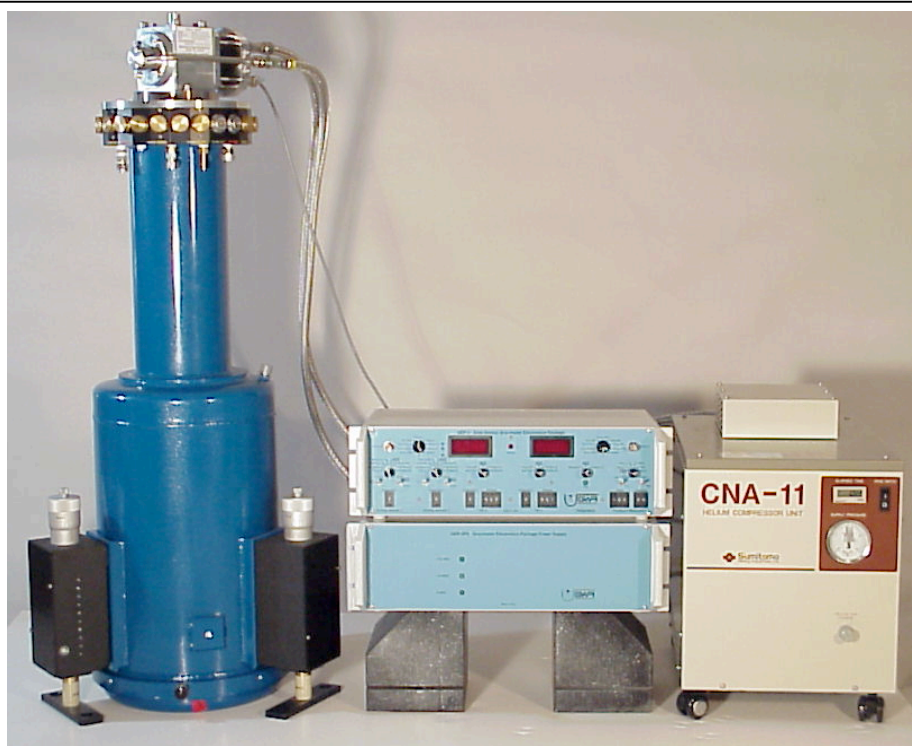
Figure 5: SG operating in a small Dewar using a Sumitomo SRDK-101 coldhead and a Sumitomo CA-11C compressor. Dewar is 10 inches in diameter and 36 inches tall
